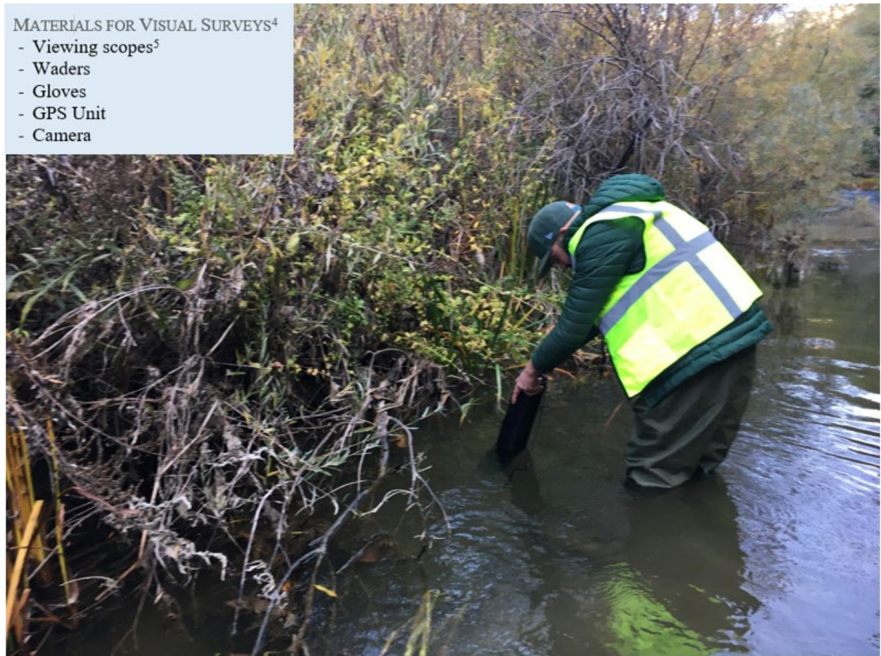
Figure 3 Drew Enstrom (ACRCD) performing visual surveys with an underwater viewing scope
